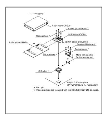
Figure 2 Usage of the R0E436049CFJ10
